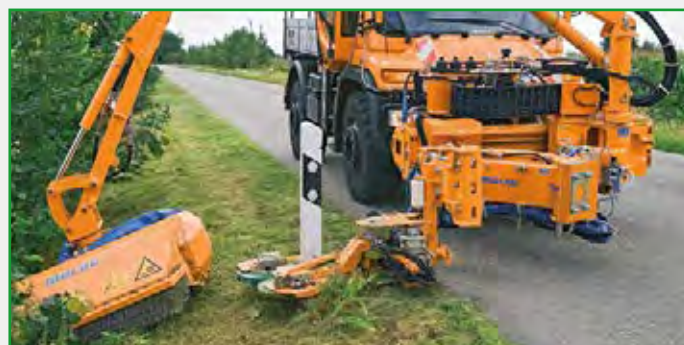
Reflexion post mower mounted on a combination mower
