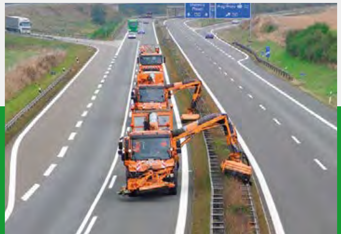
Rear-mounted mowing equipment with grass collection system
