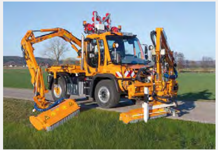
Front-mounted mowing equipment with a flexible range of applications
