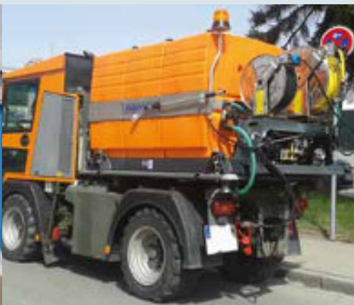
FTS 1800 with a high- and low-pressure pump
