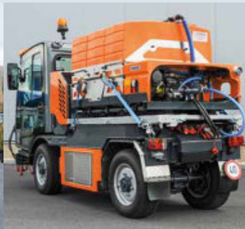
FTS 975 with a high-pressure system
