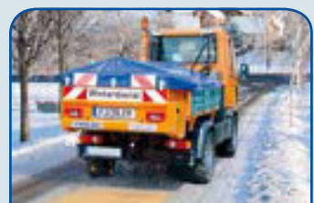
Rear mounted spreader FSH 30/30T/FWS 350/FWS 200
