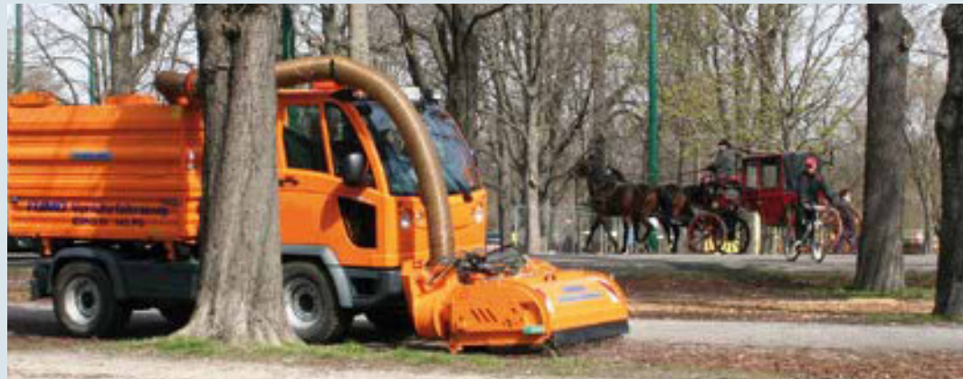
Tine harrow shaft for removing leaves and waste on sand, gravel and meadow areas
