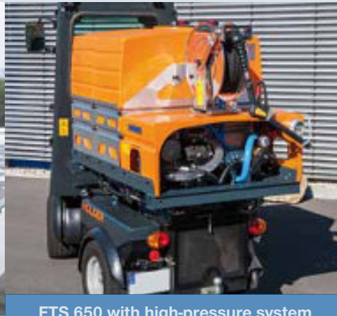
FTS 650 with high-pressure system for narrow track vehicles
