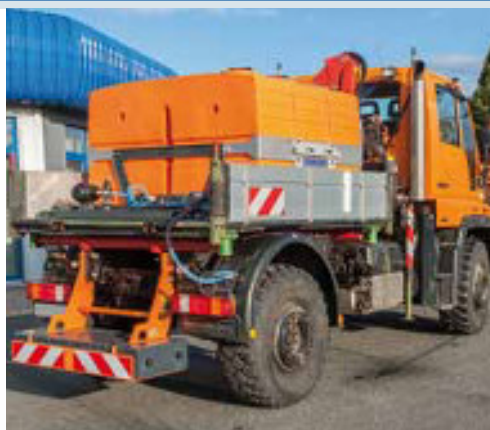
FTS 3400 with an electrical low-pressure pump
