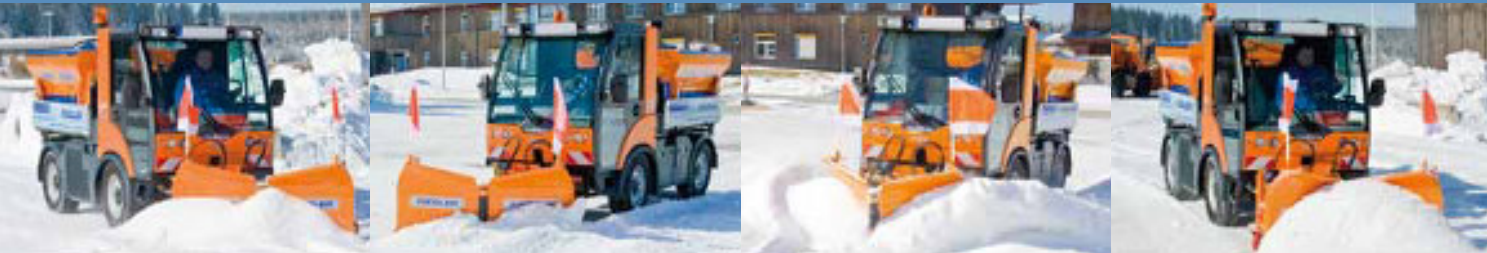
Swivels to the right as a lateral plough Swivels to the left as a lateral plough Swivels to a V – plough Swivels to a wedge plough
