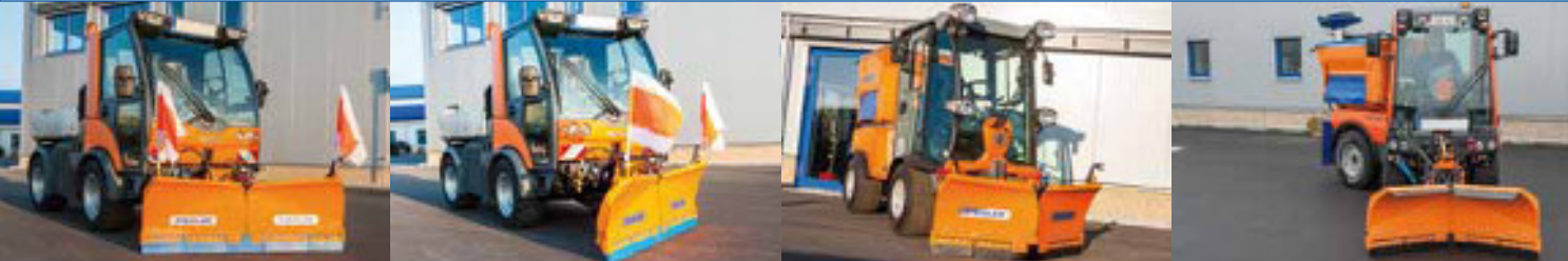
Right-hand lateral plough Left-hand lateral plough V – plough Wedge plough
