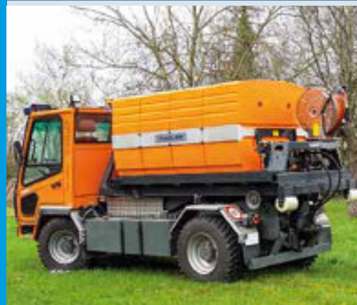
FTS 2700 with a low-pressure system on a roll-off system
