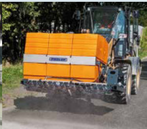
FTS 2000 with a low-pressure system for wheel loaders
