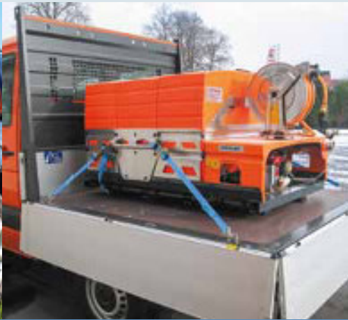
FTS 975 with a petrol engine for vans
