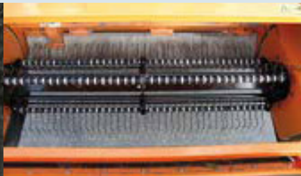
Tine harrow shaft for removing leaves and waste on sand, gravel and meadow areas
